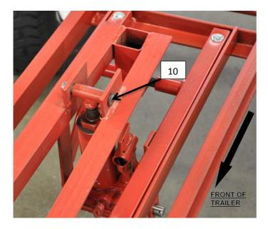
Swing slide into place over the jack, and pin in place using  $\frac{1}{2}$ " x 3-5/8" pin(10).
