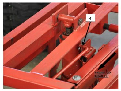
Insert the connecting rod(4) as shown into the hole on top of the jack valve and secure with cotter pin(16).
