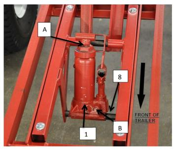
Insert jack(1) into the frame as shown in picture, using  $\frac{3}{4}$ " x 7-1/2" pin(8).
