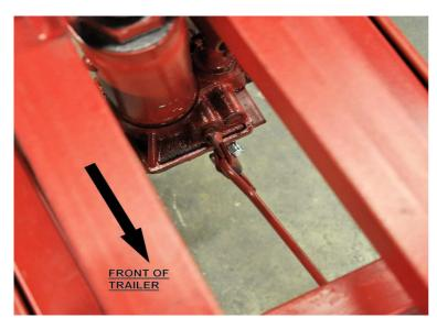
Insert the loop on the valve handle through the "U" clip(7).
