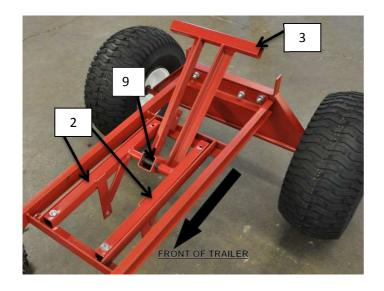
Assemble the jack frames(2), lift slide(3), and  $\frac{3}{4}$ " x 6" pin(9) as shown in picture.
