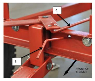
Insert the connecting rod(4) as shown and secure with cotter pin(16).
