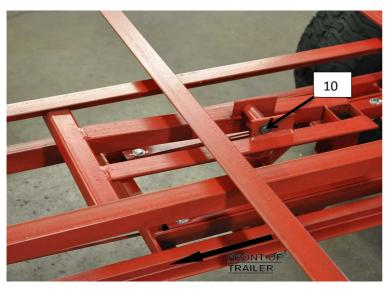
Pin bed onto frame with pin as instructed in trailer assembly.
