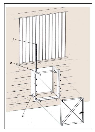
The Model CM122 Swing Out Utility Door is made so that it can swing out from either the right or left side. This is accomplished simply by inverting the unit.
