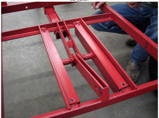
Install the bed of the trailer onto the chassis and secure the pivot pin allowing the bed to hinge up and down on the chassis. Install the upper lift arms into the upper lift bracket using the 3 inch
