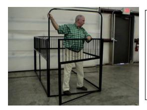
Position a modular panel on the bottom door frame hinge pin, then slowly lower the top door frame into position with the top door frame hinge sliding into the top of the modular panel frame. Make certain the top door frame side brackets slide into the top frames on the side panels.
